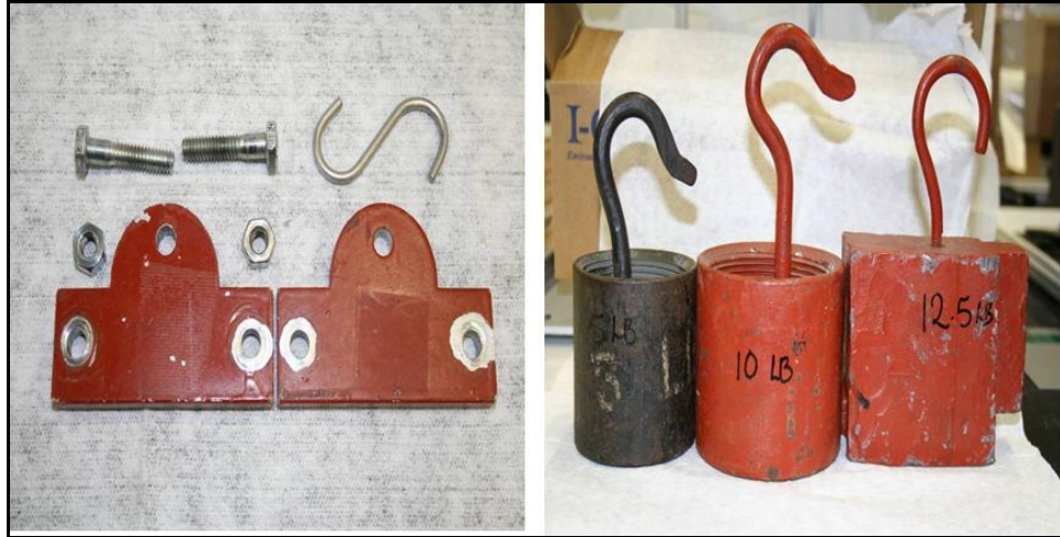
Figure 3. Clamps, screws, and bolts for strip adhesion testing (left). Weights for testing (right).
