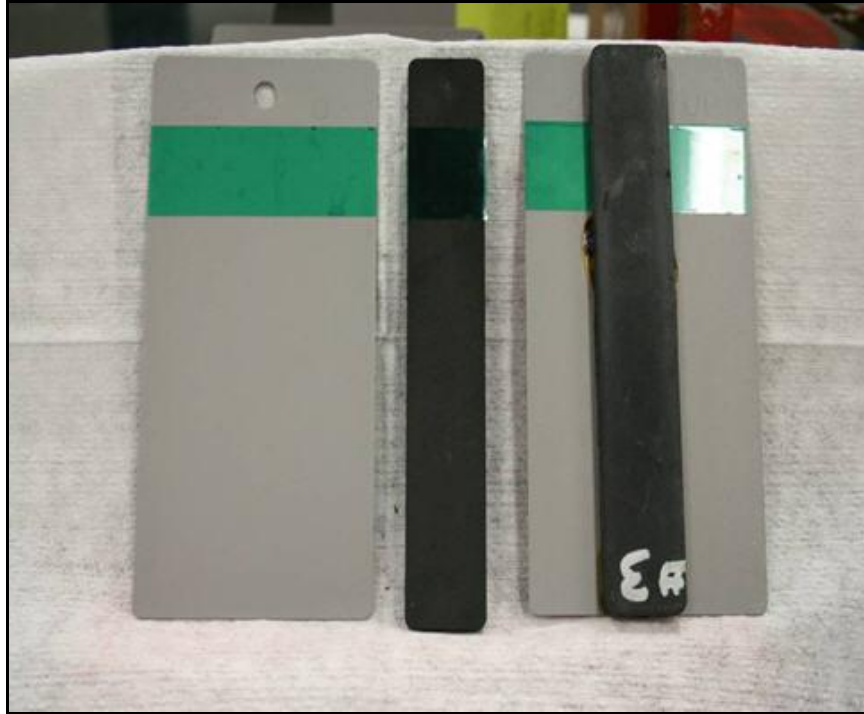
Figure 2. Steel and rubber substrates.
