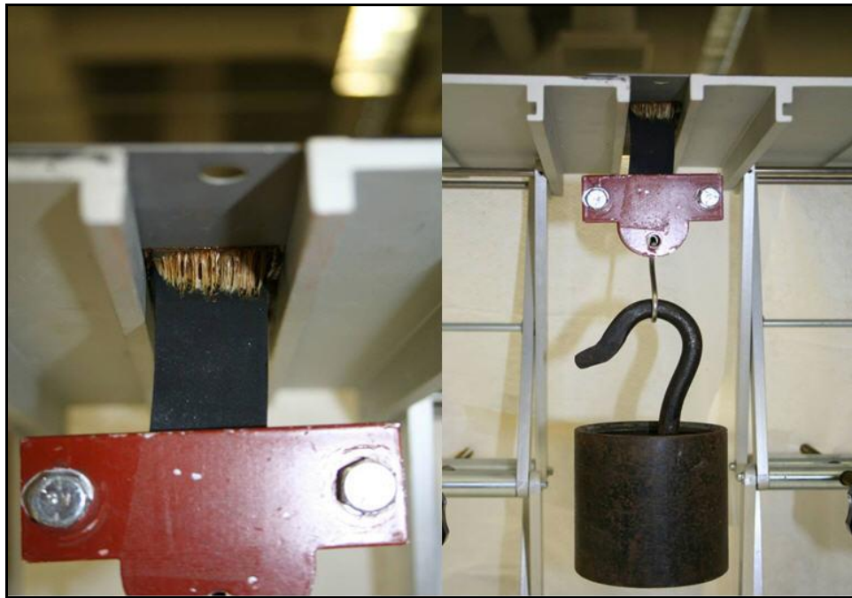
Figure 4. Strip adhesion test of the 3M-847 adhesive (left). Testing setup (right).
