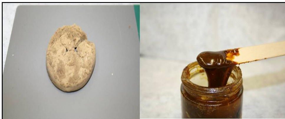
Figure 6. Sample prepared by adding dry fumed silica to adhesive (left). Successfully blended adhesive dispersion (right).
