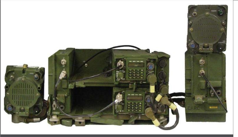
Single Channel Ground and Airborne Radio System (SINCGARS)
