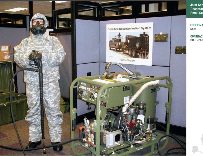
Joint Service Transportable Decontamination System (JSTDS)– Small Scale (SS)
