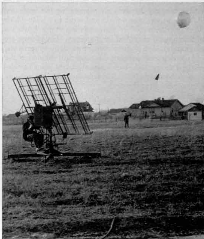
Figure 2—Radio set SCR-658 and Radiosonde, AN/AMT-2, right, rear \frac{3}{4} view, showing set tracking radiosonde prior to launching.
