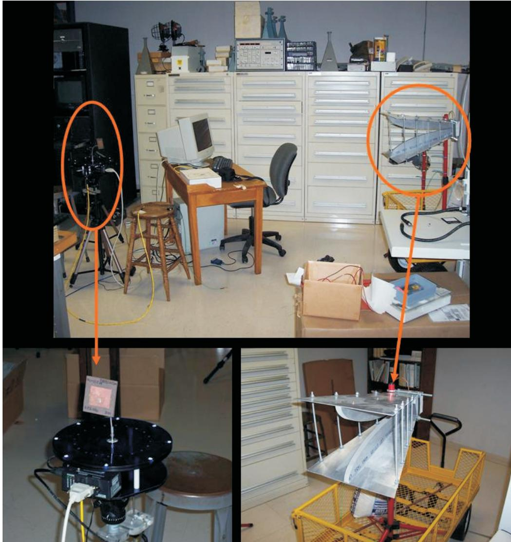
Figure 7.16: Measurement setup for antenna characterization.
