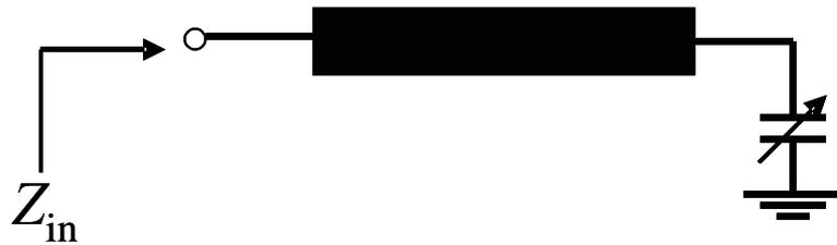
Figure 4.6: Series capacitor loaded transmission line resonator
