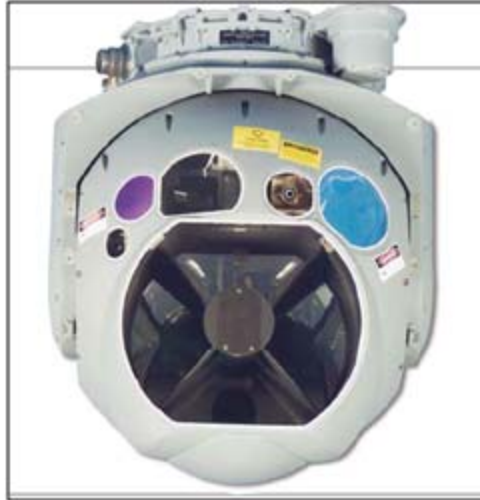
Figure 15. MTS-B FLIR System 70
