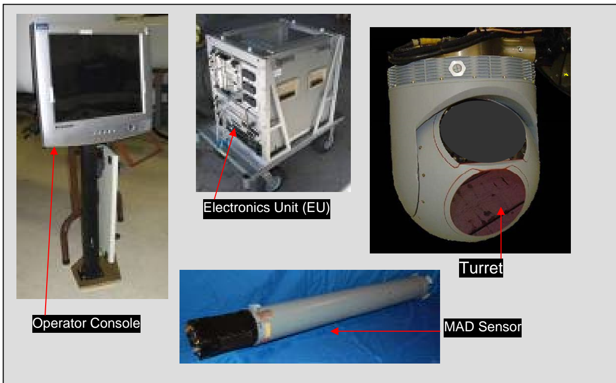
Figure 17. JMMES System Components 74
