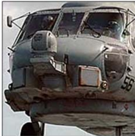
Figure 14. AAS-44 FLIR Turret onboard SH-60 Seahawk 66
