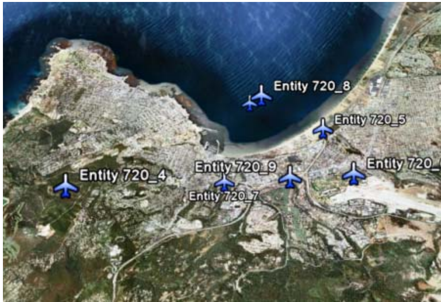
Figure 26. Screen capture showing a KML-based visualization in an Earth-browser of the entities for which the client has received state information.
