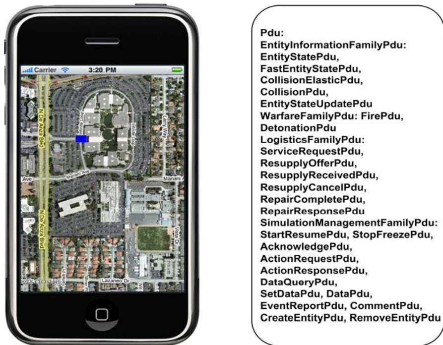
Figure 13. (l) Open-DIS running on an iPhone® controlling icon position. (r) A partial sample of the DIS PDUs implemented to date in Open-DIS.
