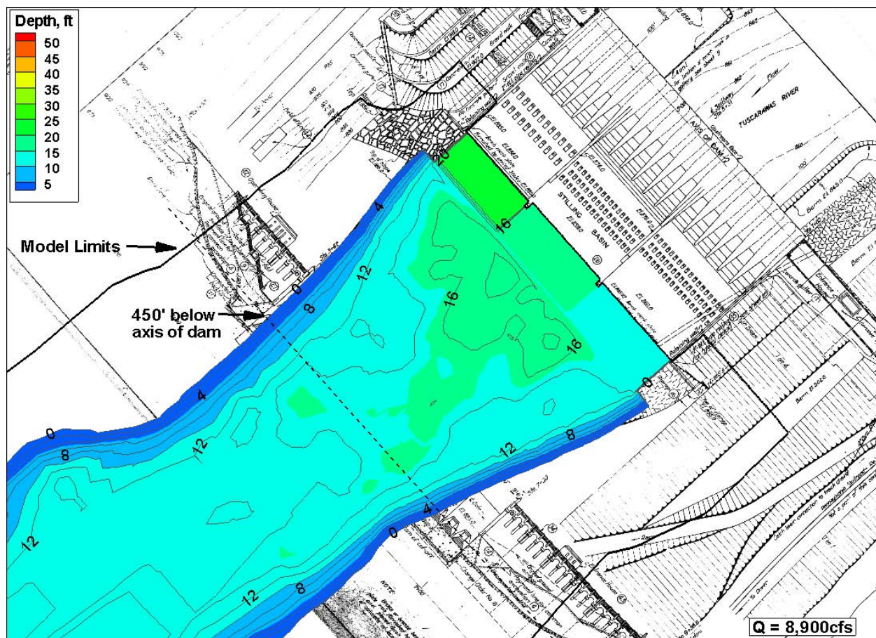
Figure 45. Water depth contours, flow Condition 7, discharge 8,900 cfs, stilling basin tailwater el 874.1.
