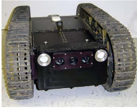
Figure 12. New URBOT sensor housing with stereo vision cameras
