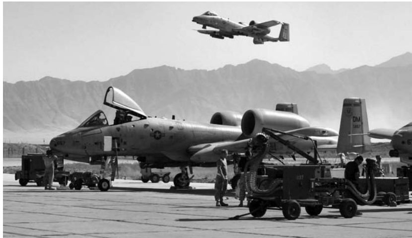
An A-10 Thunderbolt II takes off on a combat mission as A-10 crew chiefs, weapons loaders, and an avionics specialist ready others for another mission. The A-10 was the first Air Force aircraft designed for close air support of ground forces.
