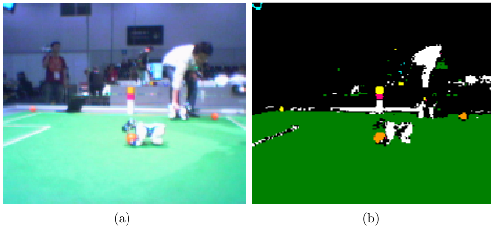
Figure B.3: Example vision data from the AIBO camera. (a) The original image. (b) The color segmented image.
