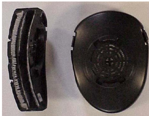
JSGPM 2 JSGPM/M50 Filter - note the curved shape and filtration materials
