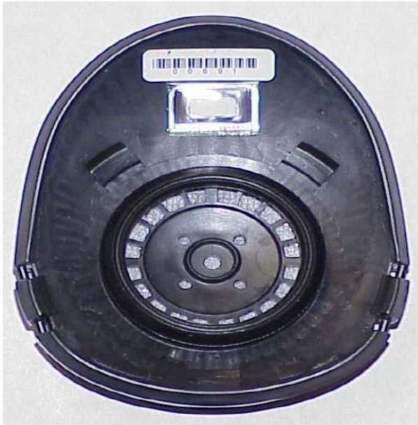
JSGPM 3 JSGPM/M50 Filter - note the clip locks on the side and the bayonet ring in the middle that opens the receiver on the mask. This closes when the filter is removed, limiting contamination during filter exchanges.
