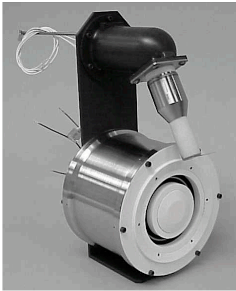
Figure 1. Photograph of Busek Co., Inc. circular BHT-600 Hall thruster. Photograph courtesy of the Busek Company, Natick, MA.
