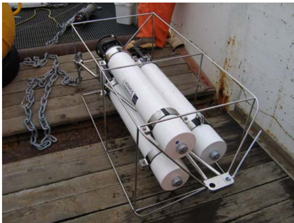
Figure 2. Left: image of three-frequency AWCP trio mounted in reinforced stainless steel mooring cage. Right: image of AWCP sensors and PAL being deployed at mooring site M2.
