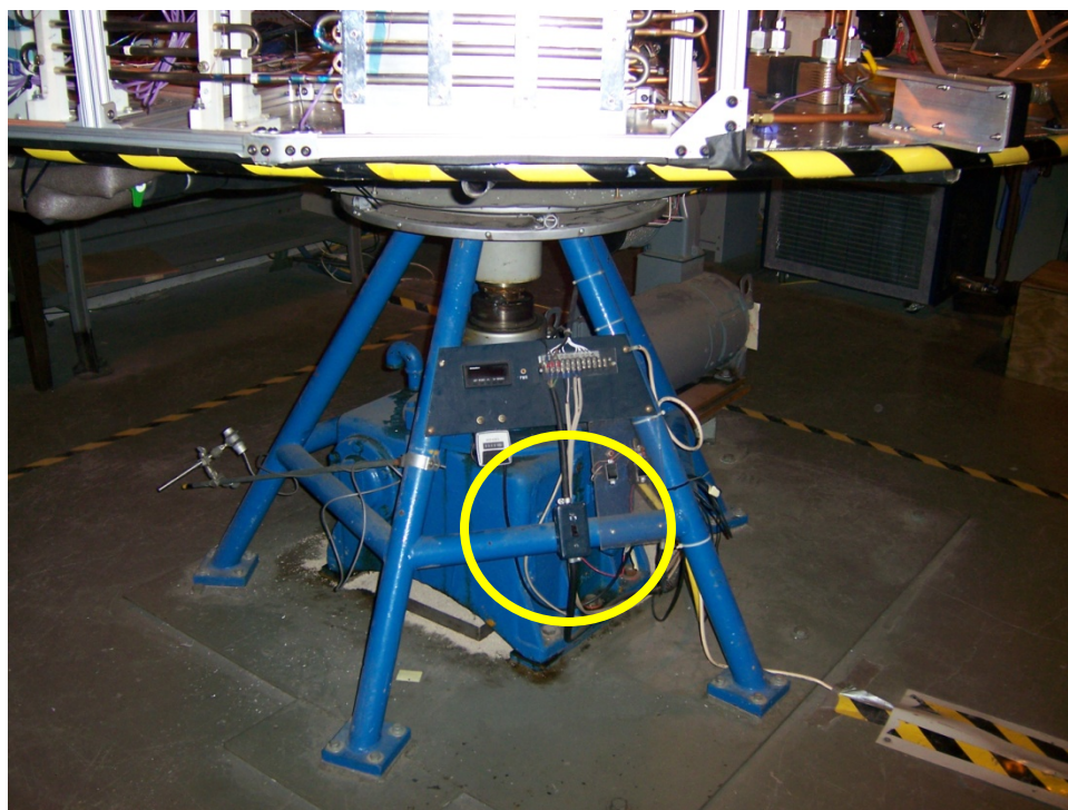
Figure A.4. Centrifuge table power switch.
