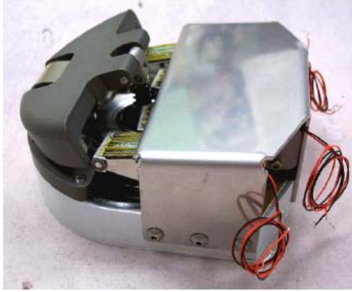
Fig 1: Proof of Concept Heel Strike Generator [2]
