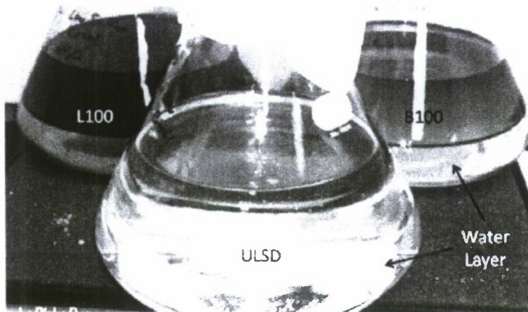
Figure 1. Image of the pre-exposure fuels L100, ULSD, and B100 and distilled water layers.
