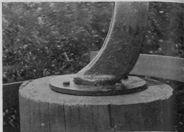
Socket and shank of machine-gun yoke.
