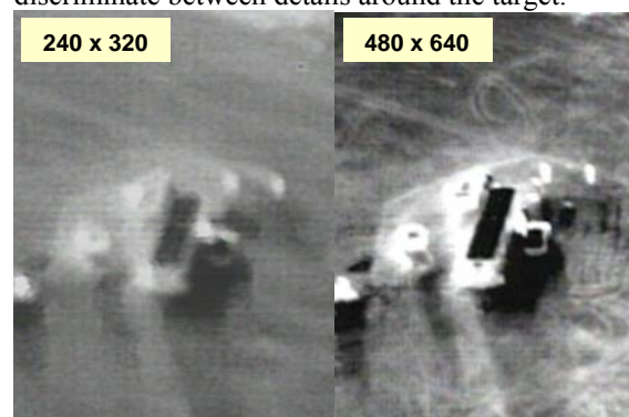
Figure 2. IR video frames collected simultaneously at 1000 feet above ground level (AGL). These images clearly identify improved detail (including tyre tracks) at the higher resolution.
