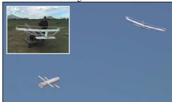
Figure 7. Configuration One - Airborne gradiometer with the Silver Fox mounted transmitter and a towed, air core gradiometer. Insert shows transmitter.
