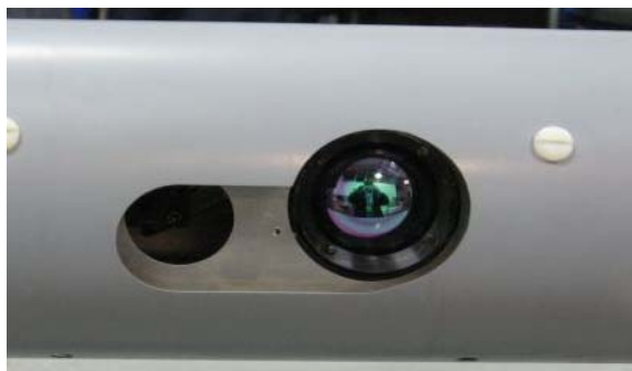
Figure 3. Camera mounts on the B4 Silver Fox UAV for the low and higher resolution IR video cameras.
