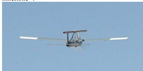
Figure 12. Gradiometer configuration on the Silver Fox UAV used for tunnel detection.
