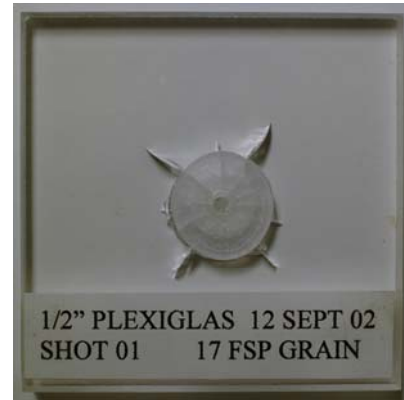
Figure 7: Experimental impact at 1004 m/s
