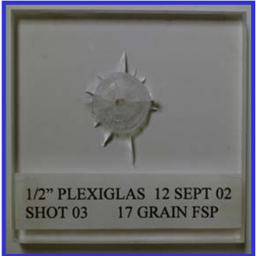
Figure 5: Experimental impact at 846 m/s
