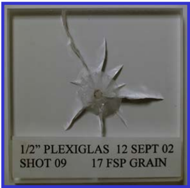
Figure 3: Experimental impact at 475 m/s
