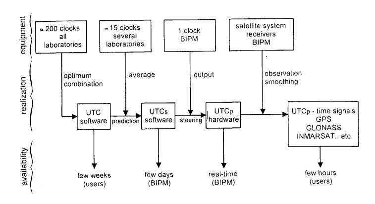
Figure 1. Block diagram of the realization of the real-time prediction of UTC, UTCp
