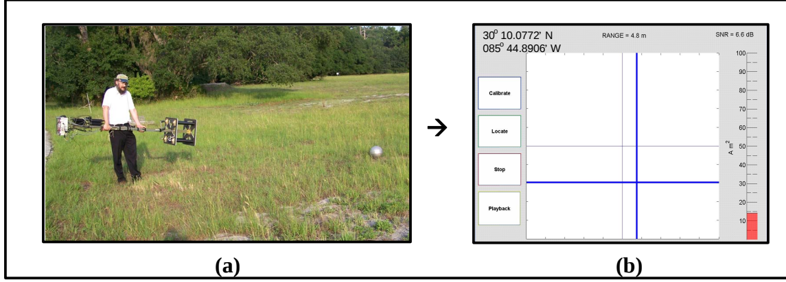
FIG. 1. Prototype MagSTAR Sensor and screenshot of near real time DLC data.
