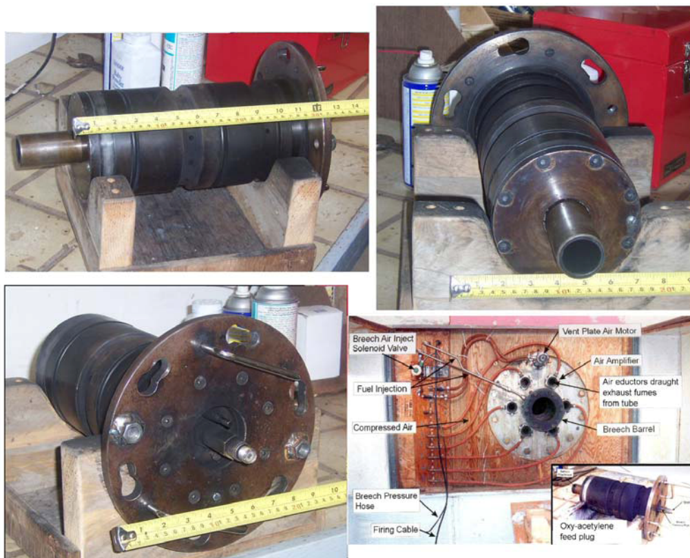
Figure 7. Current removable breech plug for mounting of FAE initiator balloon.
