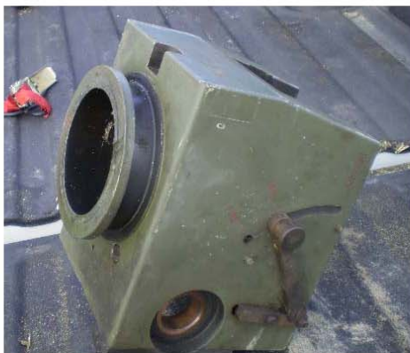
Figure 9. Breech for the 76mm cannon certified for firing blank ammunition which can be reconfigured as an interim driver for the Blast Tube.
