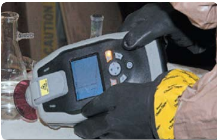
Ahura: The portable, cutting-edge Ahura provides effective HME identification for warfighters in Iraq and Afghanistan. JIEDDO Photo
