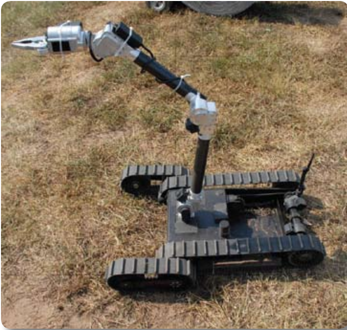
MARCBot/XBot: Omnipresent on the battlefield, military robots like the XBot continue to serve a vital role in IED detection and neutralization. JIEDDO Photo
