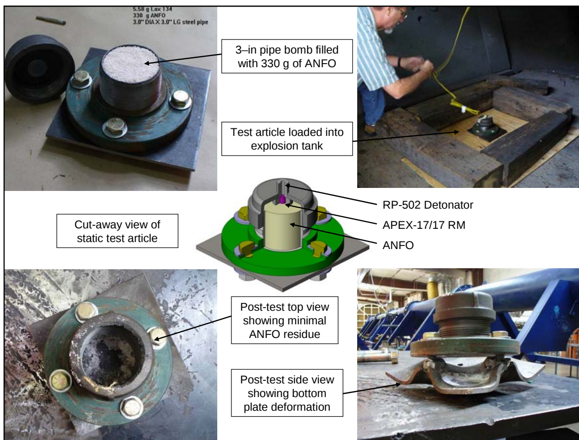
Figure 4.1. Three-inch pipe bomb test article.
