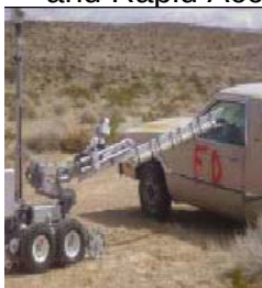
RANT being positioned by robot inside car
