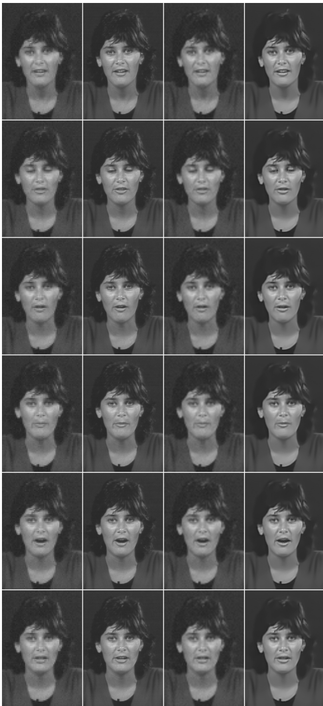
Fig. 8. Results for the 3rd, 8th, 13th, 18th, 23rd, and the 28th frames from the “Miss America” sequence. From left to right: Low resolution image; original image (ground truth); Lanczos interpolation; result of the proposed algorithm.
