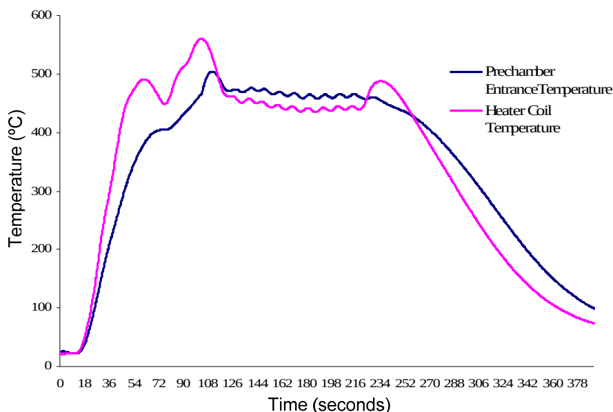
Figure 3.9: Temperature control during cold spray deposition
