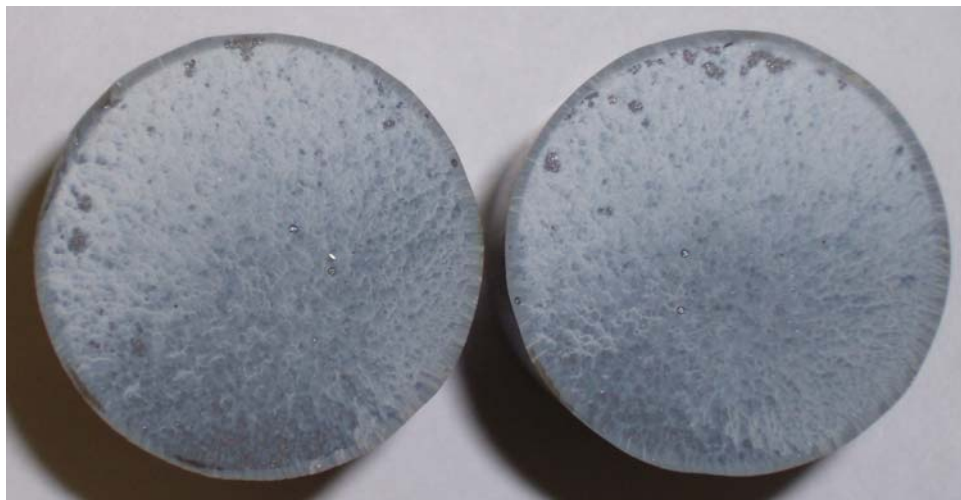
Figure 4-41: Fractured surface of HYSOL epoxy as a result of bond testing
