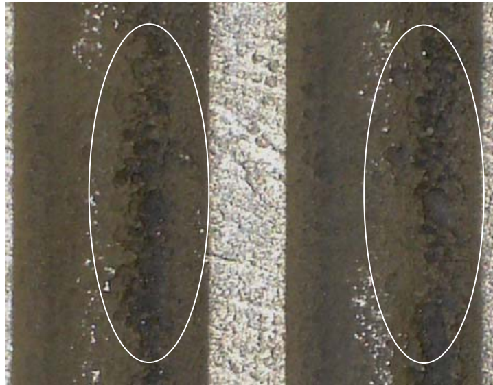
Figure 5.11: Top view of an as-sprayed Ni-7 wt% MoS 2 coating using milled feedstock showing erosion of coating by subsequent passes
