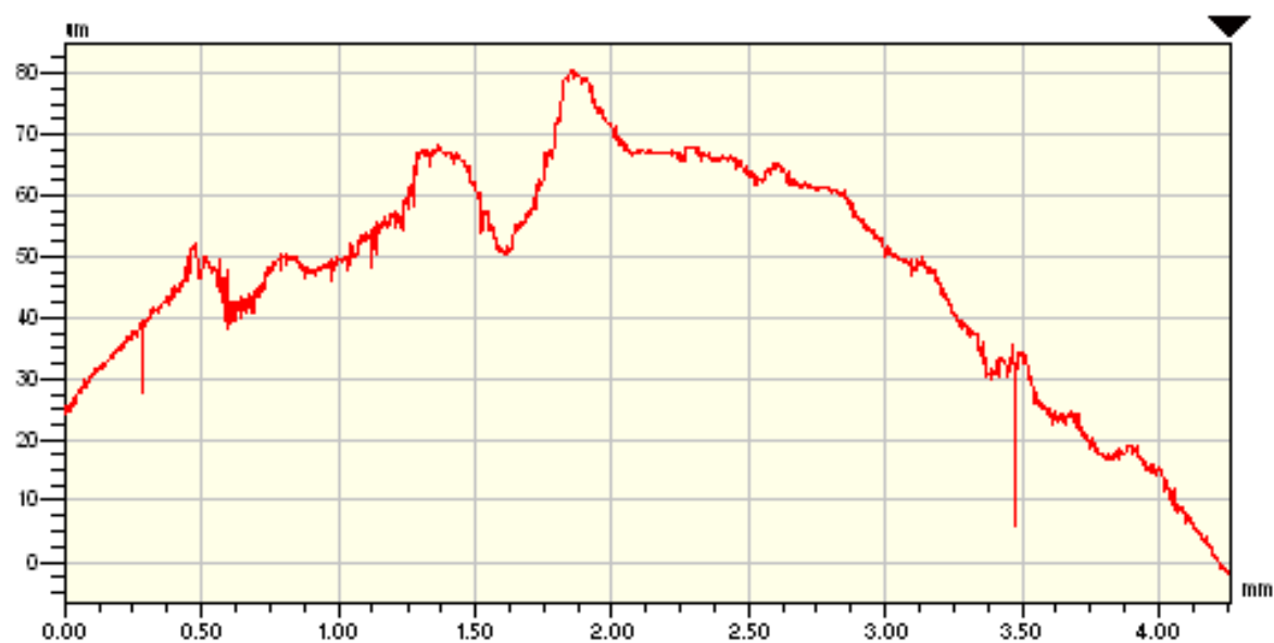
Figure 5.42: Wear trace of the uncoated Ti-6Al-4V ellipse worn against the machined Ni-30 wt. % Ni coated BN coating along the major axis
