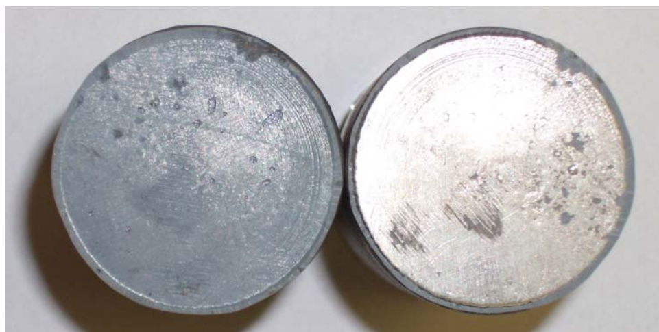
Figure 4-42: Fractured surface of the pure Ni cold spray coating as a result of bond testing
