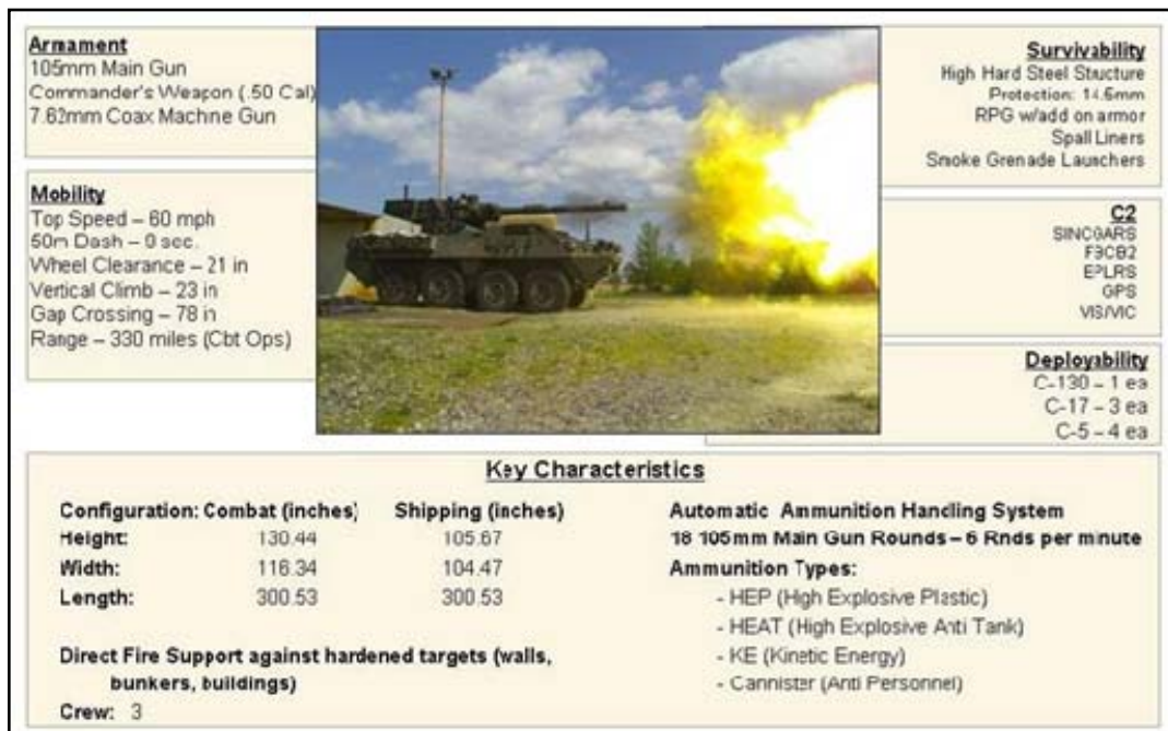
Figure 5. Mobile Gun System Characteristics (From McCarroll, 2008, slide 37)
