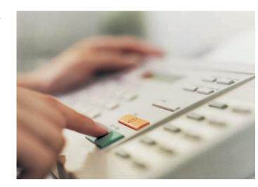
**NSTS**: NSA/CSS Secure Telephone System (NSTS) is a stand-alone secure telephone system that allows conversation up to the TS-SCI level. IC entities call these phones by different names, such as grey, white, or green phones, although these colors do not always reflect the actual color of the telephone unit.
