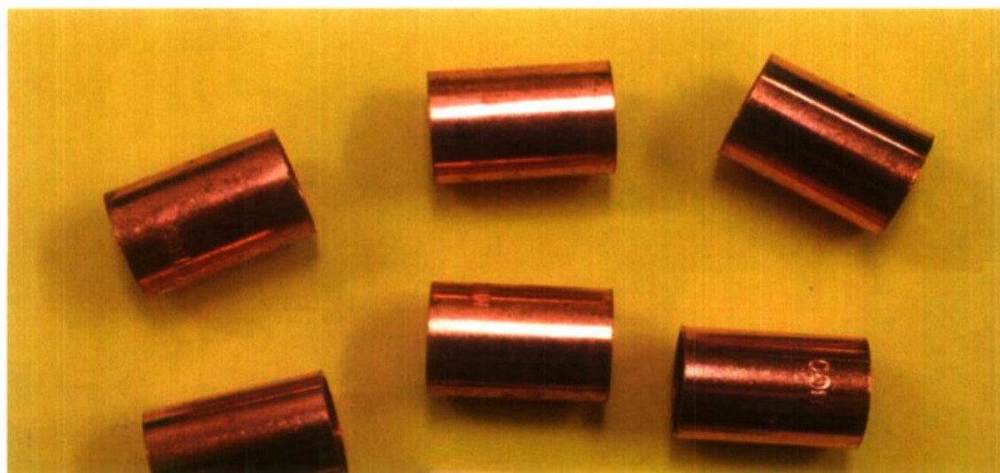
Figure 12. Photograph of copper tubing prior to exposure to \text{ClO}_2 .
