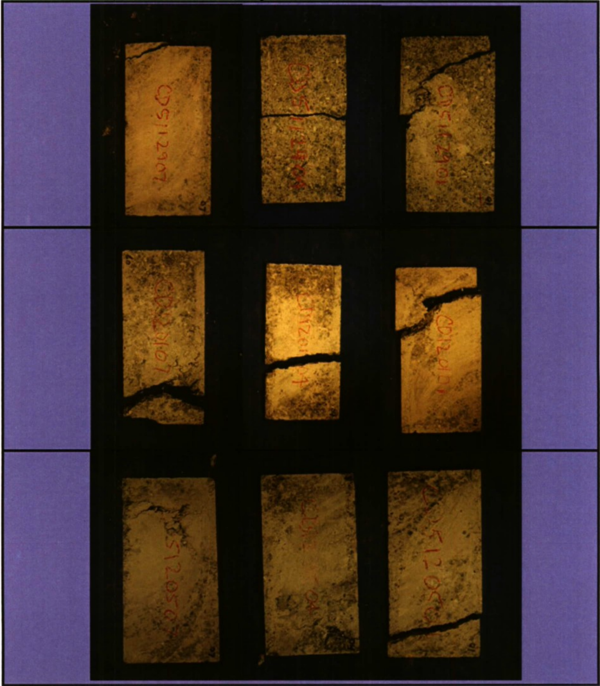
Concrete cinder block coupon location of break: ClO 2 control set
