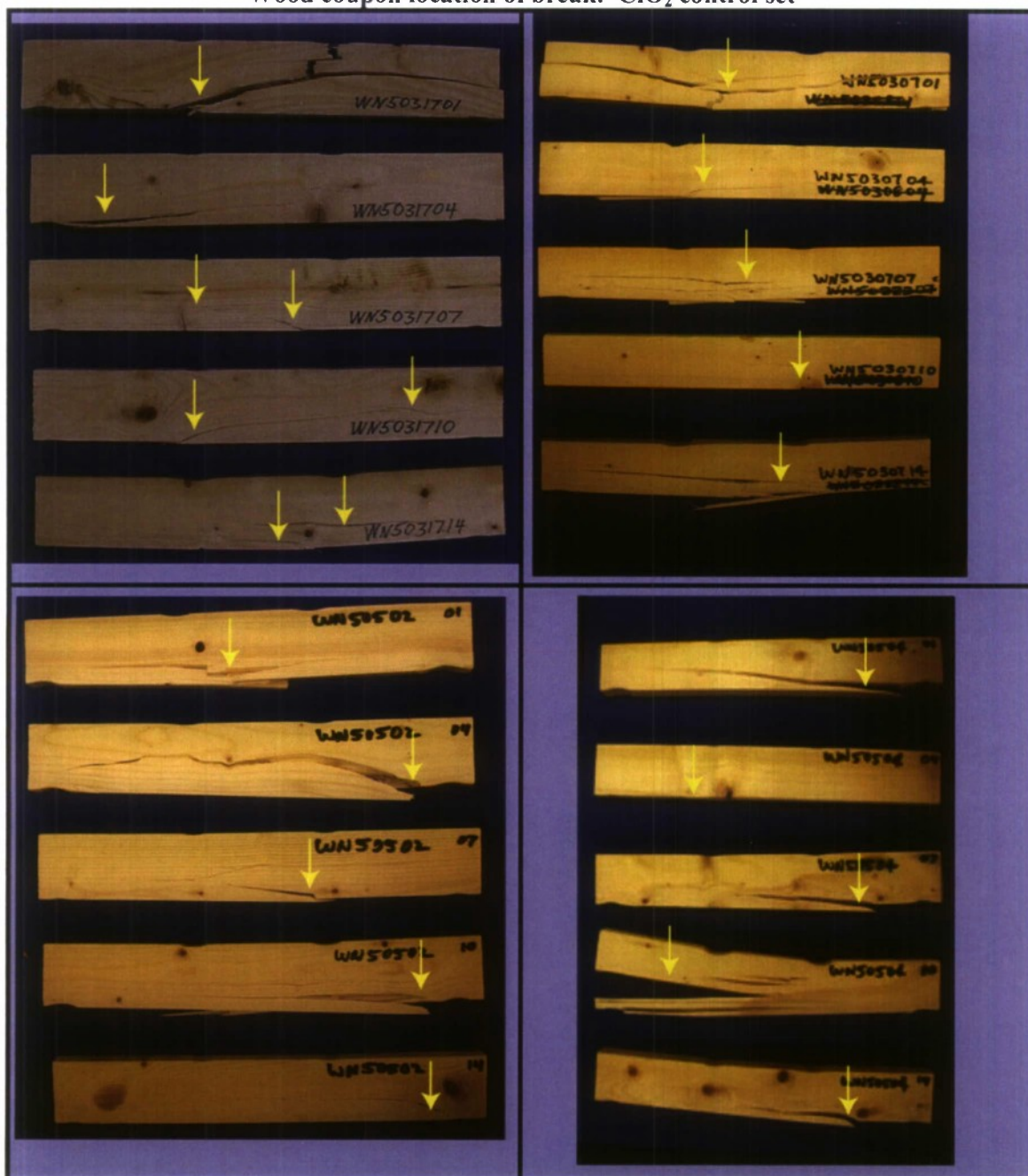
Wood coupon location of break: ClO 2 control set
