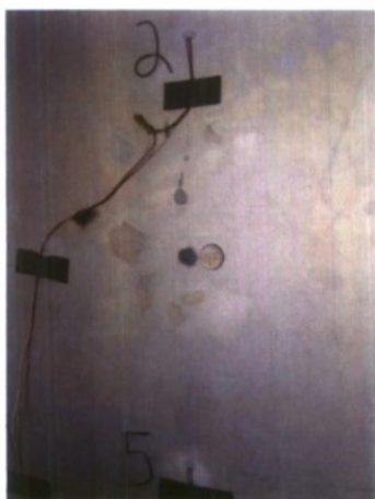
Figure 24 Saltwater corrosion spots around damage 1.
