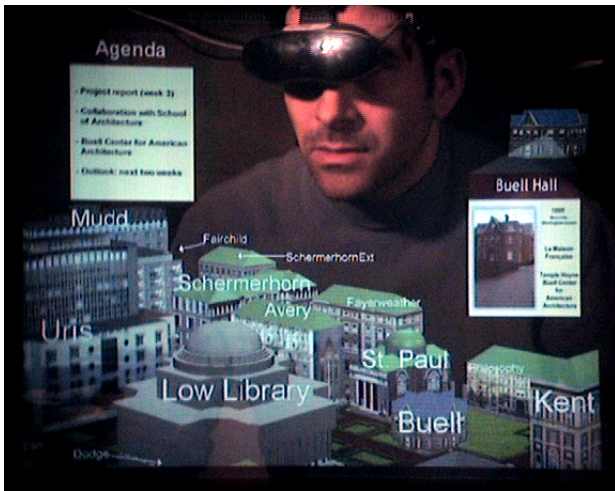
Figure 10: View management in a collaborative system (imaged through see-through head-worn display). Labels are laid out dynamically to annotate the buildings of a campus model as seen by the observer. UI elements avoid overlapping the colleague's head and the campus model.
