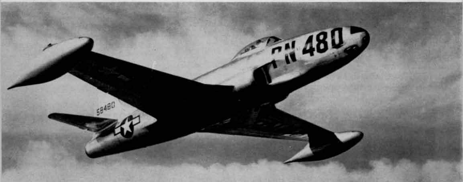
F-80B, Lockheed's "Shooting Star," has also been thoroughly tested in operations over Korea. It is in the 600 mph class at altitudes of over 45,000 feet armed with rockets and machine guns.
