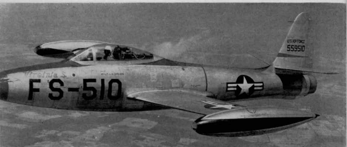
Republic F-84 Thunderjet: First American jet fighter to fly over 600 miles an hour with a service ceiling of 45,000 feet, the Thunderjet is armed with six caliber .50 machine guns and can carry a substantial rocket load for ranges up to 850 mph.
