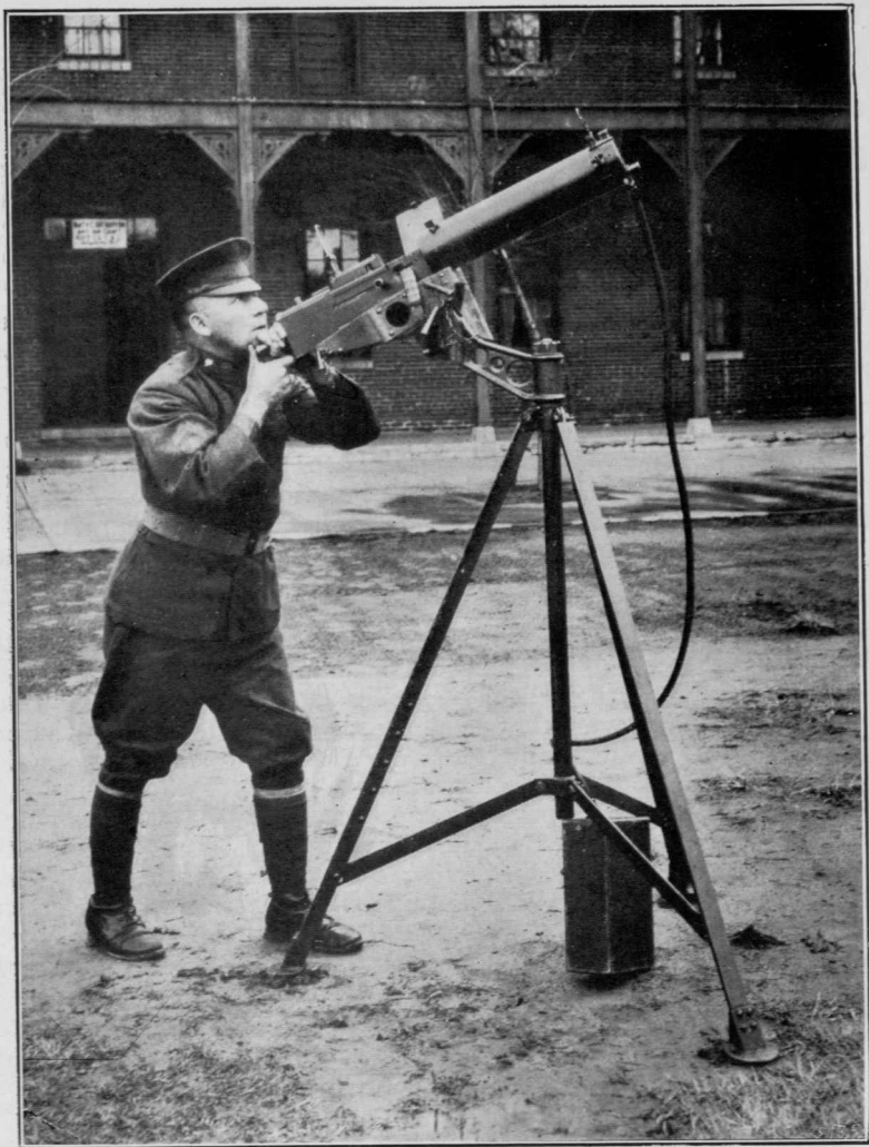
FIG. 1. .30 CALIBER BROWNING MACHINE GUN, MODEL 1917, MOUNTED ON ANTI-AIRCRAFT TRIPOD, MODEL 1918
