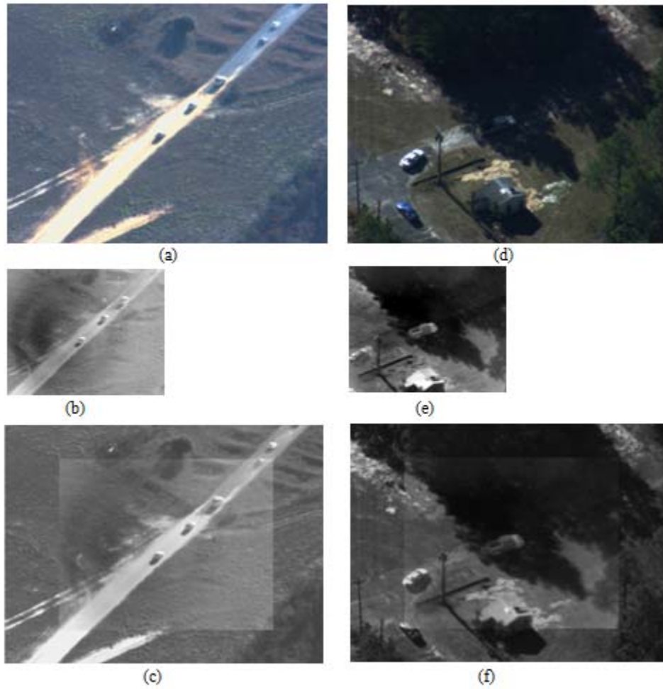
Fig.6. Image fusion results (a) Optical image; (b) IR image; (c) Fusion of image in (a) and (b); (d) Optical image; (e) IR image; (f) Fusion of image in (d) and (e).
