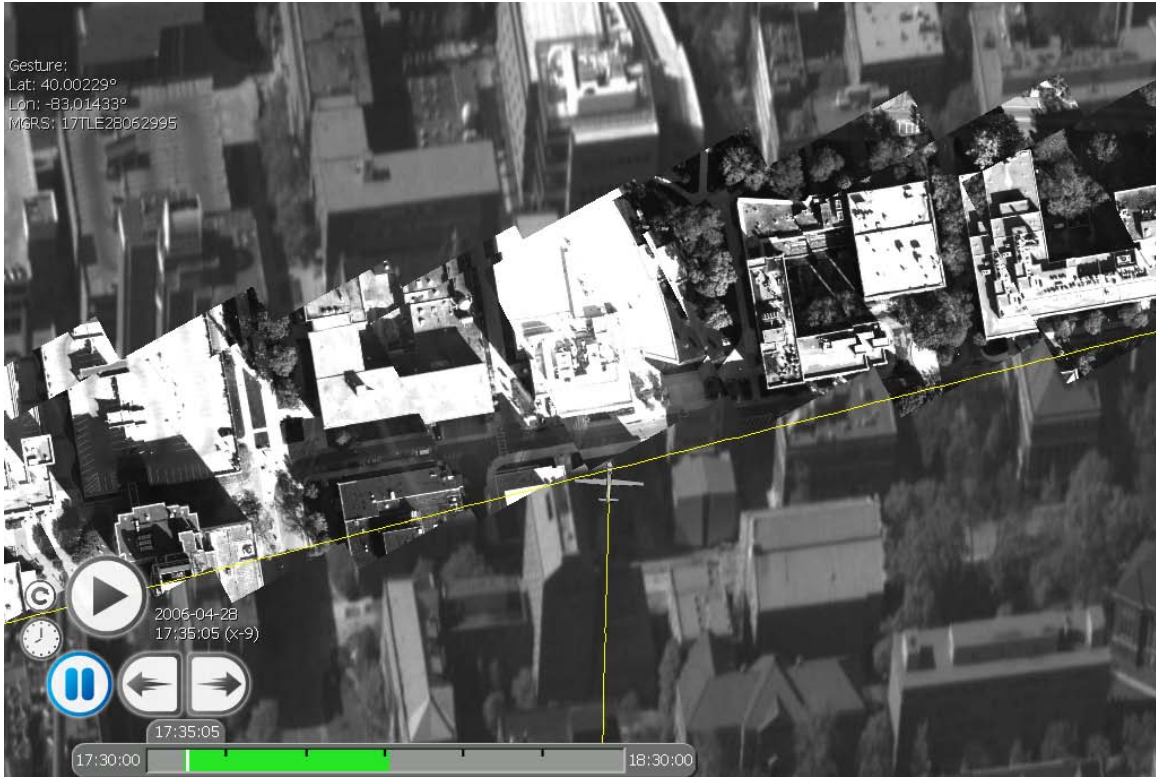
Figure C.2: Pictured here is an illustration of fused electro optical and synthetic aperture radar imagery.
