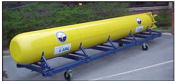
Figure 1. The Seahorse AUV constructed for the Naval Oceanographic Office
