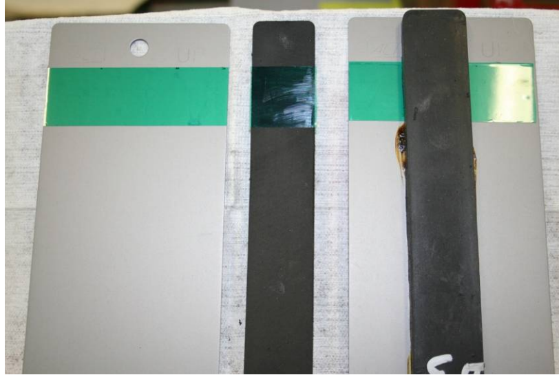
Figure 1. Basic assembly for strip adhesion.
