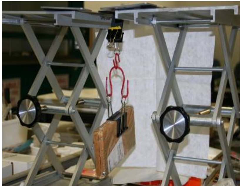
Figure 2. Basic strip adhesion setup for MMM-A-121.
