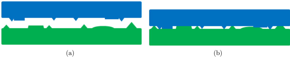
Figure 2.4: Example of surface roughness (a) which leads to a decreased contact area at pull-in (b).
