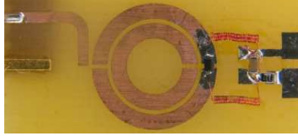
Figure 2.29: Varactor-loaded SRR system along with circuitry used for voltage biasing [48].
