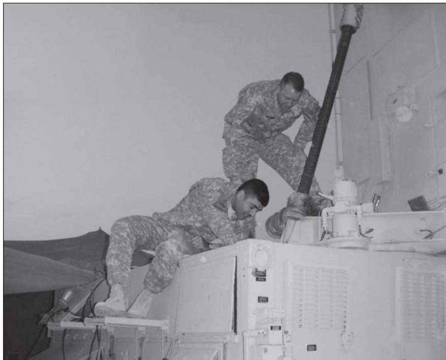
Chief Warrant Officer Two (CW2) Jasbir Riat and Sergeant Don Grainger from D/1-94 FA troubleshoot a Q-37 Firefinder radar in Iraq.
