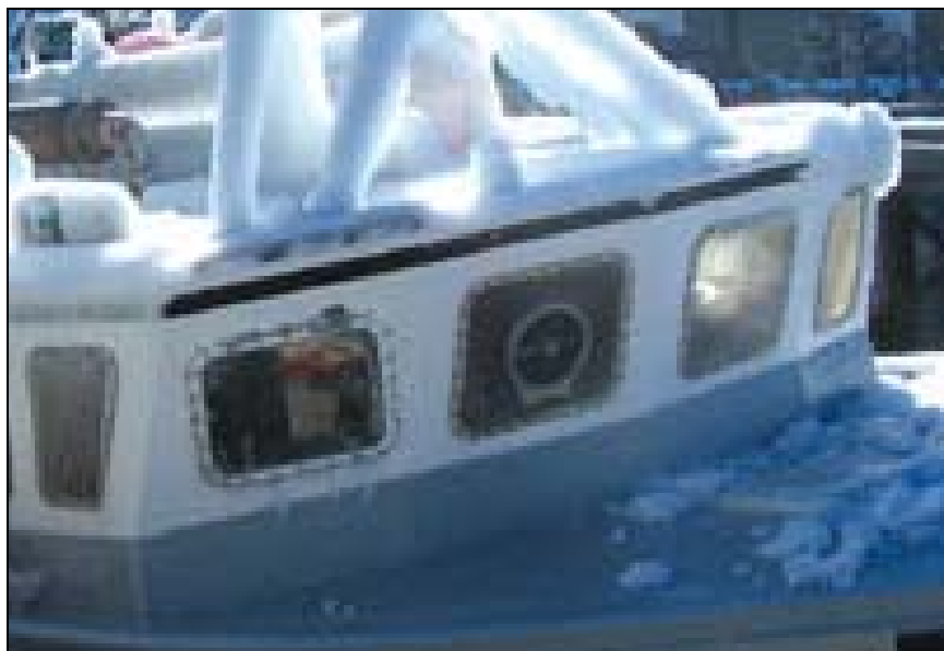
Figure 49. Typical spinning window used to keep ship bridge windows dry and free of ice on Navy ships. Viewed from inside the bridge (top). Spinning window mounted on small supply boat (bottom).
