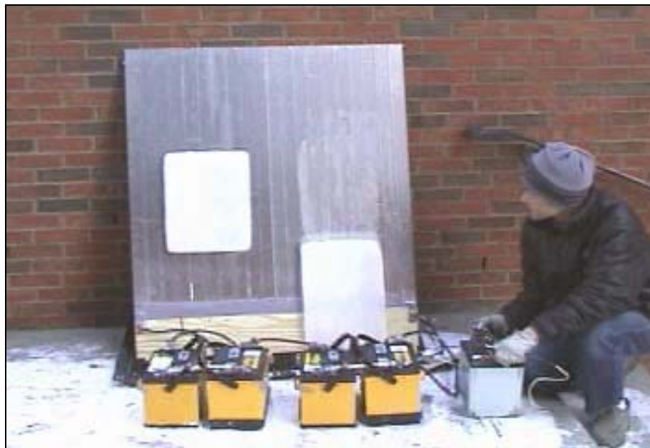
Figure 26. Deicing a metal plate with pulse electrothermal deicing. The ice sheet on the right was released moments before the image frame was acquired.
