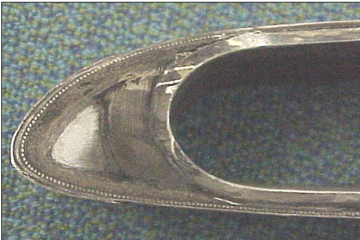
Figure 33. Cross section of Black Hawk helicopter blade showing the ends of heater wires immediately under the leading edge wear strip.
