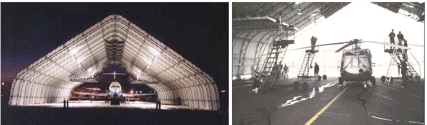
Figure 42. Radiant Aviation Services system for deicing aircraft (left), and in use for experimentally deicing Army helicopters (right).
