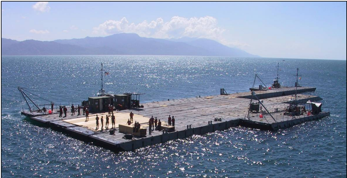
Figure 10: MCS units acting as RO/RO discharge facility
