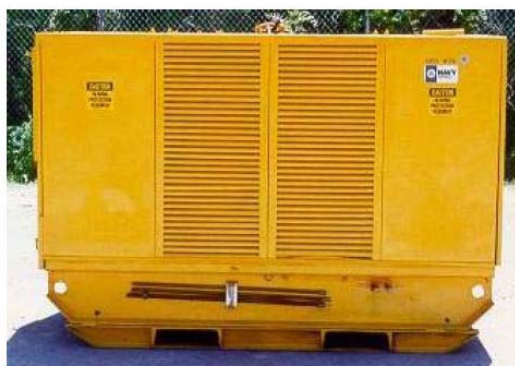
Figure 17: ESSM 30 kW Diesel Generator
