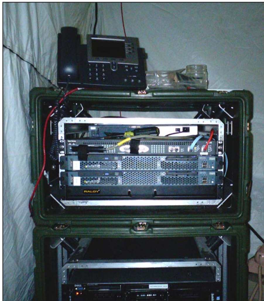
(Above left) Access Layer Network Case photo: An Access layer transit case for the III Corps TAC command post is displayed. This setup for a switch and an UPS is standard for delivery network connectivity to all our subscribers.
