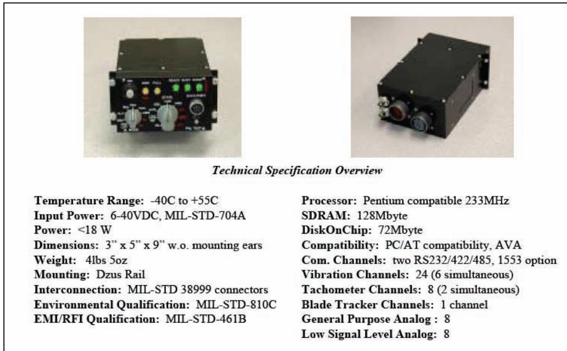
Figure 2.21. Technical specification of the HUMS box for the VMEP.
