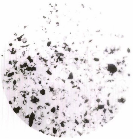
Fig.19. CG 34 X50 M889 Wet incorporation of 12.5% powdered graphite.
