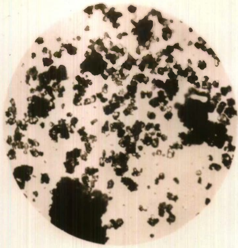
Fig.1. CG3 X50 M855. Graphited R.D.1303. 1% gelatin 3.7% colloidal graphite.
