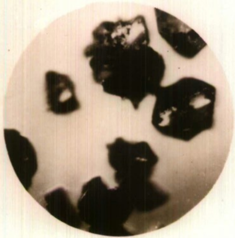
Fig.3. CG19 X280 M852. Enlarged crystals of graphited RD.1303 showing partial coating.
