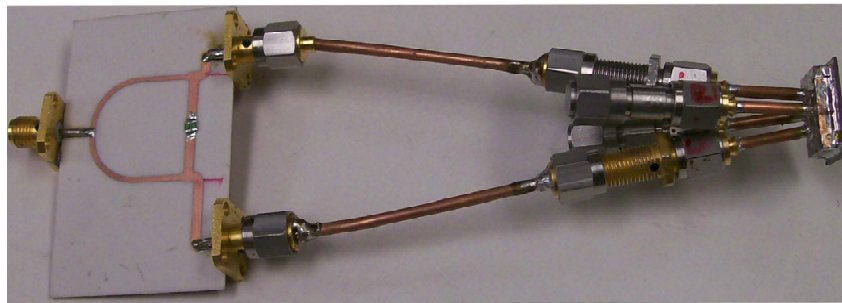
Figure 7: X-Band DFCBSA prototype including power divider.
