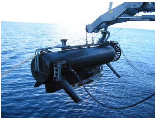
Figure 5: Deploying Snorkeler Class USV (Program Executive Officer, Littoral and Mine Warfare. The Navy Unmanned Surface Vehicle (USV) Master Plan [23 July 2007]: cover)
