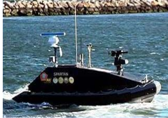
Figure 4: Spartan Scout USV (Program Executive Officer, Littoral and Mine Warfare. The Navy Unmanned Surface Vehicle (USV) Master Plan [23 July 2007]: 6)
