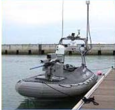
Figure 3: Example of Harbor Class USV (Program Executive Officer, Littoral and Mine Warfare. The Navy Unmanned Surface Vehicle (USV) Master Plan [23 July 2007]: 38)
