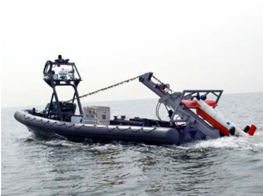
Figure 7: Fleet Class USV with Tow Gear (Program Executive Officer, Littoral and Mine Warfare. The Navy Unmanned Surface Vehicle (USV) Master Plan [23 July 2007]: cover)
