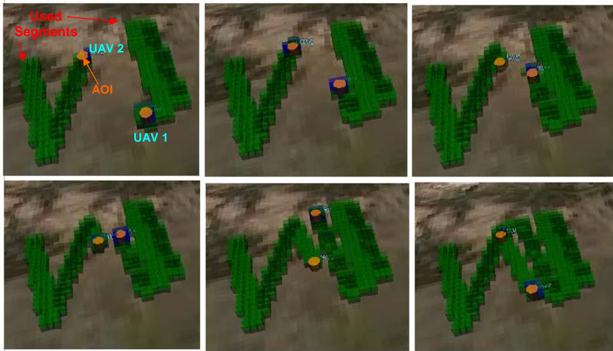
Figure 27: Scenario of two UAVs creating paths as they traverse in a designated polygonal airspace (filtered from display)
