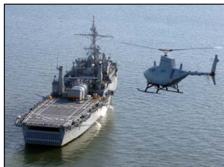
An RQ-8A Fire Scout (Group 4 UAS) Vertical Takeoff and Landing Tactical Unmanned Aerial Vehicle (VTUAV) System prepares to land aboard the amphibious transport dock ship USS Nashville (LPD 13).
