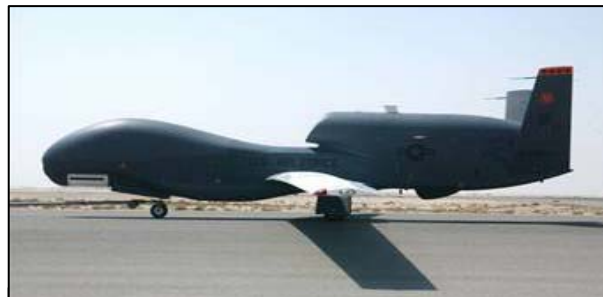
An RQ-4 Global Hawk (Group 5 UAS) unmanned aerial vehicle is towed back to its hangar following a mission at a deployed location in Southwest Asia. The Global Hawk requires access to all classes of airspace for the conduct of operational and training missions.
