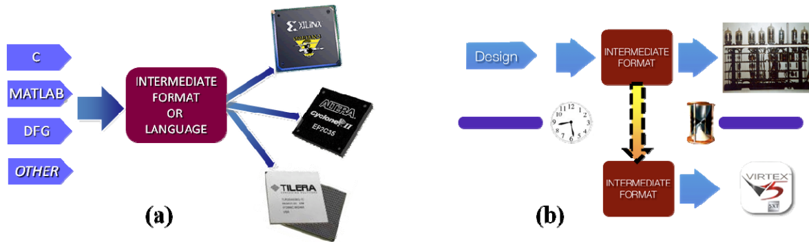
Figure 4: Two Key Benefits of Hardware Reuse: (a) The Ability to Retarget other Devices, and (b) Mitigation of Obsolescence.
