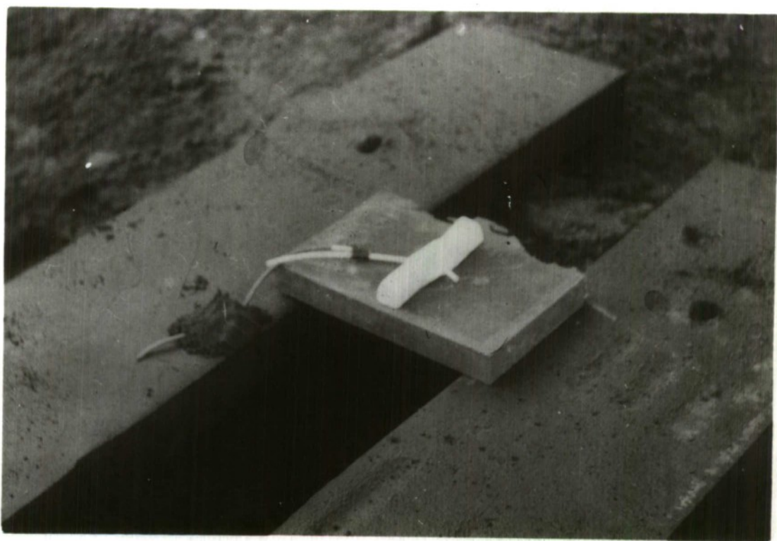
Photo No. 10. Initiation by detonating cord of cartridge on 1\frac{1}{2} " witness plate
